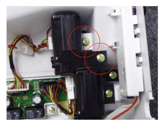
7. Using your screwdriver, wiggle/pry the hinge/motor out of position.
