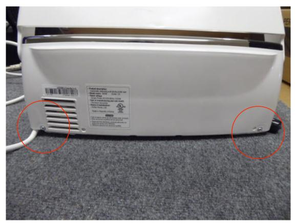
4. Locate the six pry locations in the lower housing. Insert a flat blade screwdriver and gently pry the upper and lower housing apart.
