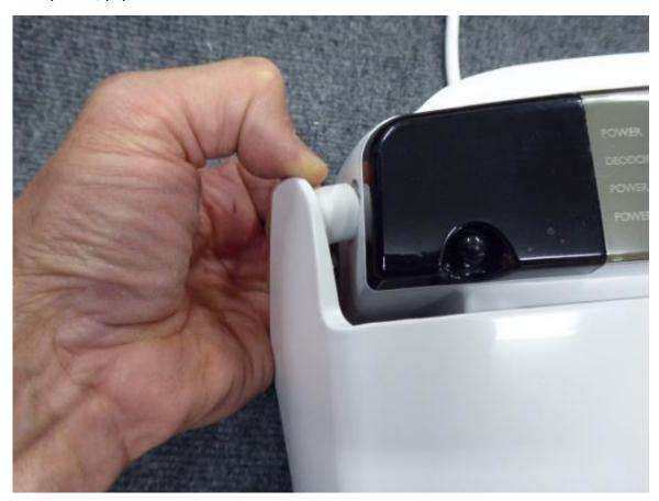
2. Wiggle and push the lid towards the right to disengage the cam on the right side.
