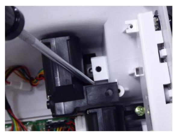
8. Note the hinge pin is a cam (oblong) shape and must match up with the bushing on the seat when reinstalling.
